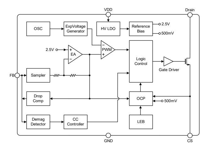
Figure 2.Block diagram of SP2689FC
