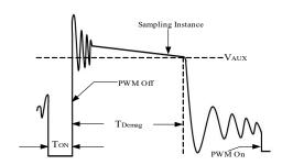
Figure 4. Auxiliary voltage waveform
