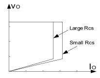
Figure 5.Adjustable output power by changing Rs
