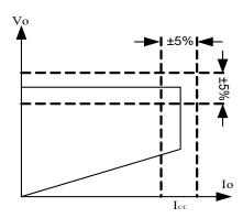
Figure 3. Typical CC/CV Curve
